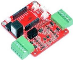
The **BOKRA I2C 4AI ADS1x15 Pro** modules are professional analog input modules based on 16-bit ADS1115 and 12-bit ADS1015 ADC. Compatible with most types of microcontrollers (I<sup>2</sup>C interface is used to communicate with them).
