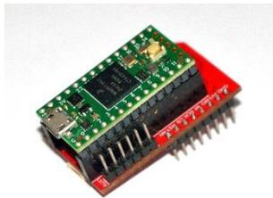
The **Teensy Shield** is an adapter that allows you to install [Teensy 4.0](#), [Teensy 3.2](#), [Teensy LC](#) and previously produced [Teensy 3.1](#) modules in the mikroBUS slot or connect mikroBUS modules (such as [MikroElektronika](#)'s Click®) to Teensy modules.
